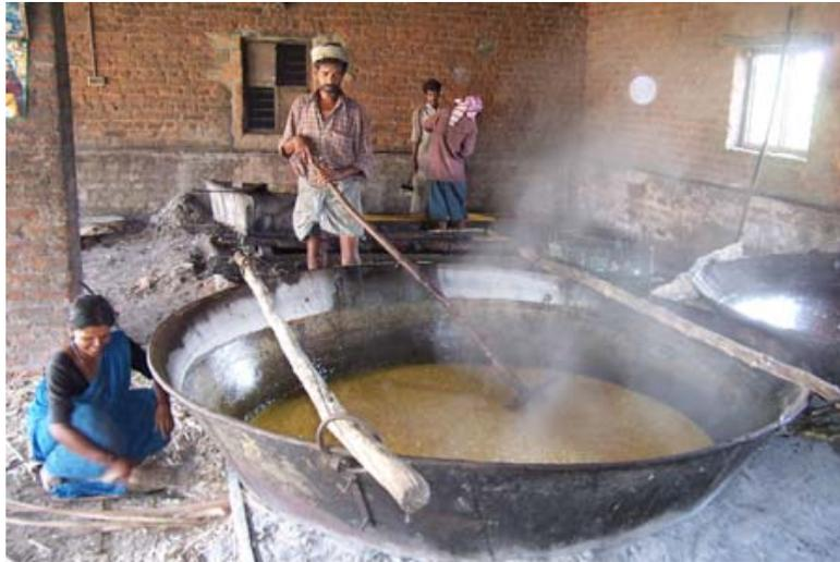
difficulty with most of common furnaces is their excessive fuel consumption and low rate of boiling. Boiling of juice to the proper consistency requires great skill on the part of the boiler as slight over-boiling results in caramelization and consequent damage to the colour and flavour of the **gur**.
